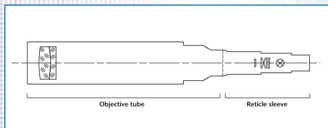
A measuring unit for tilt angles can be built by combination of a collimator with a telescope, when there is a need to measure in transmission.
